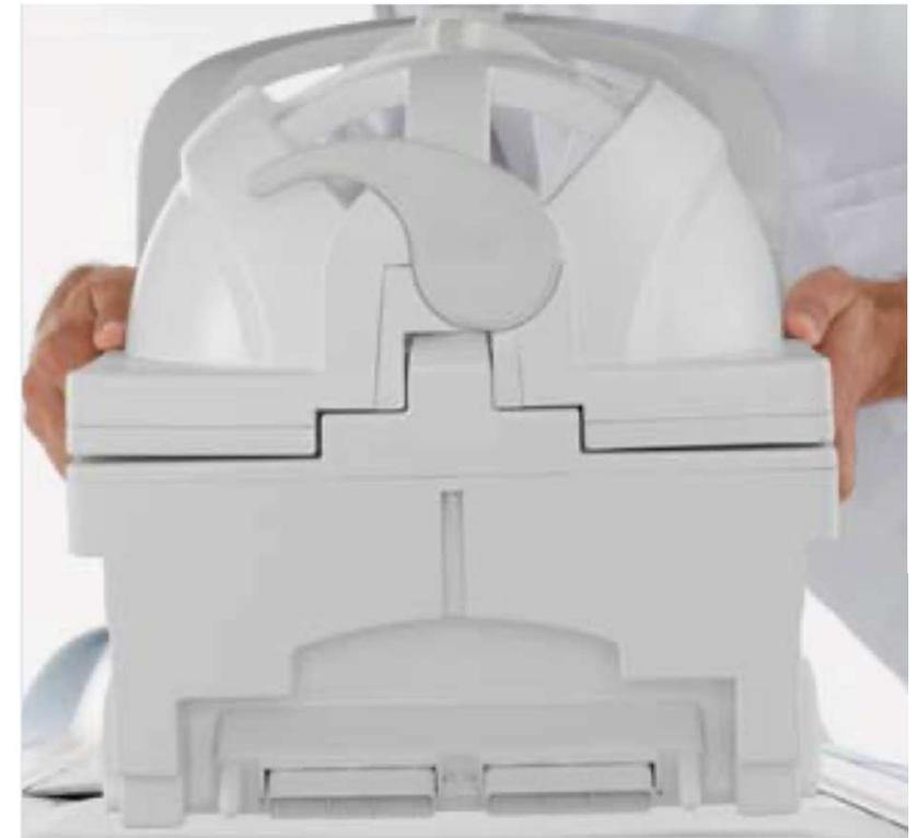
**New DirectConnect coils.** Eliminate the hassle and inefficiency of cables. With no attenuating cable, you'll also enjoy an improvement in SNR.
