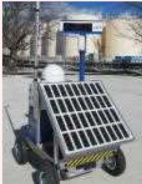
Installation of Dose-rate monitor
