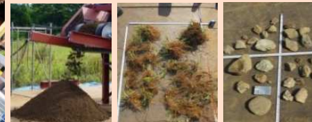
Picture 2 - results of foreign material removal by R/S (left: soil, center: light material, right: heavy material)
