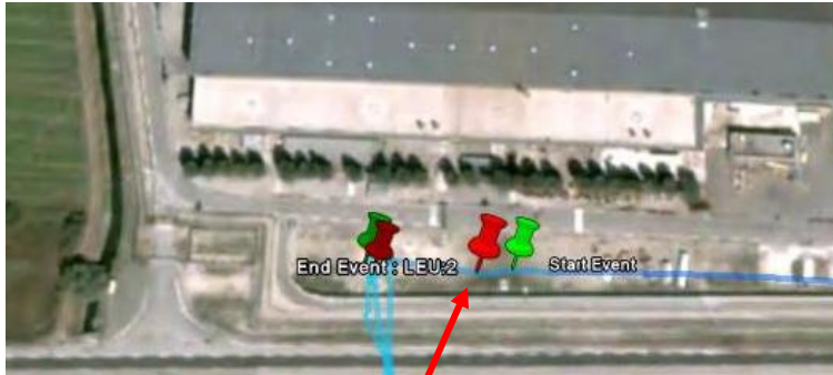
Weak LEU identified in 2 seconds from road passing by an enrichment facility
