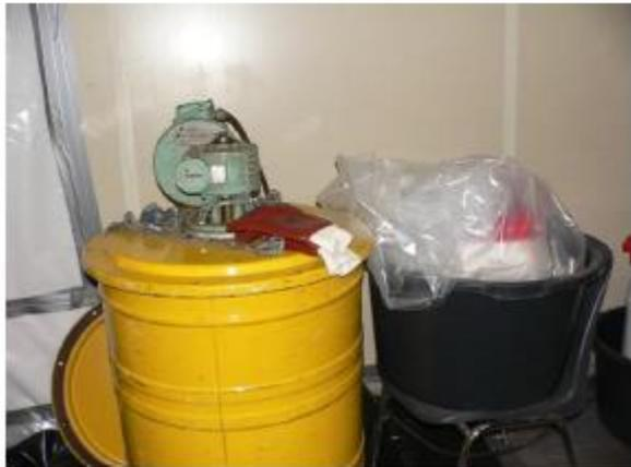
Fig. 6.3. Yellow dust barrel with stirring device.
