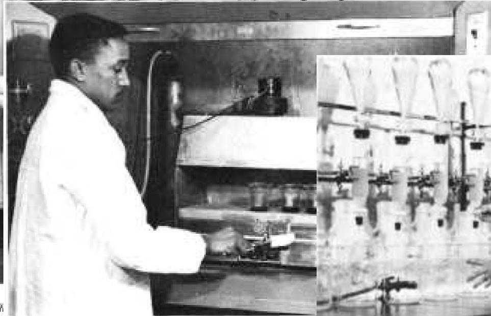
A chemist separates strontium-90 as a solution from a solution prepared from milk rated prior to counting.
