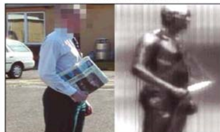
Spot the knife? Millimeter waves, close to terahertz, show their ability to see through clothes and paper.
